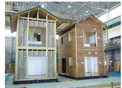
Testing at the National Research Institute for Earth Science and Disaster Prevention using a full-scale vibration table. This testing has proven the superb earthquake proofing performance of Dailite.
