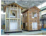
Testing at the National Research Institute for Earth Science and Disaster Prevention using a full-scale vibration table. This testing has proven the superb earthquake proofing performance of Dailite.
