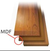
MDF      | <b>建材・家具の基材</b><br>(ドア、収納、窓枠等の芯材)<br>
